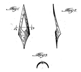
Figure 1 is a front elevational view of a pen point or similar article showing our new design;
