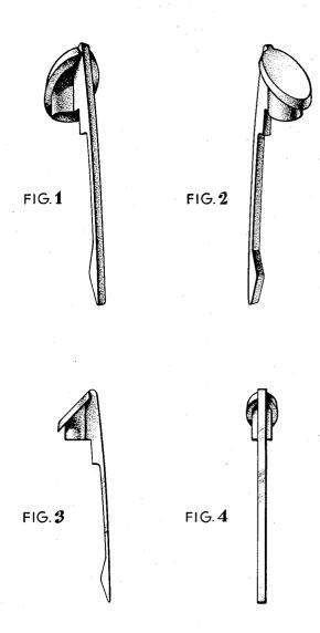
Fig. 1 is a front perspective view of a clip for a fountain pen or similar article showing my new design;
