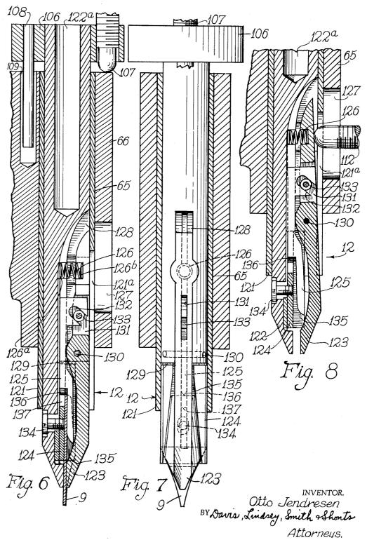
APPARATUS FOR TIPPING METAL BASES WITH METAL TIPS
